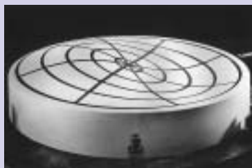
FIGURE 8.21 A marked rubber “drumhead” vibrating in several of its possible modes. Here we see side-by-side pairs of still photographs from three of the symmetrical modes and from an anti-symmetrical mode.
