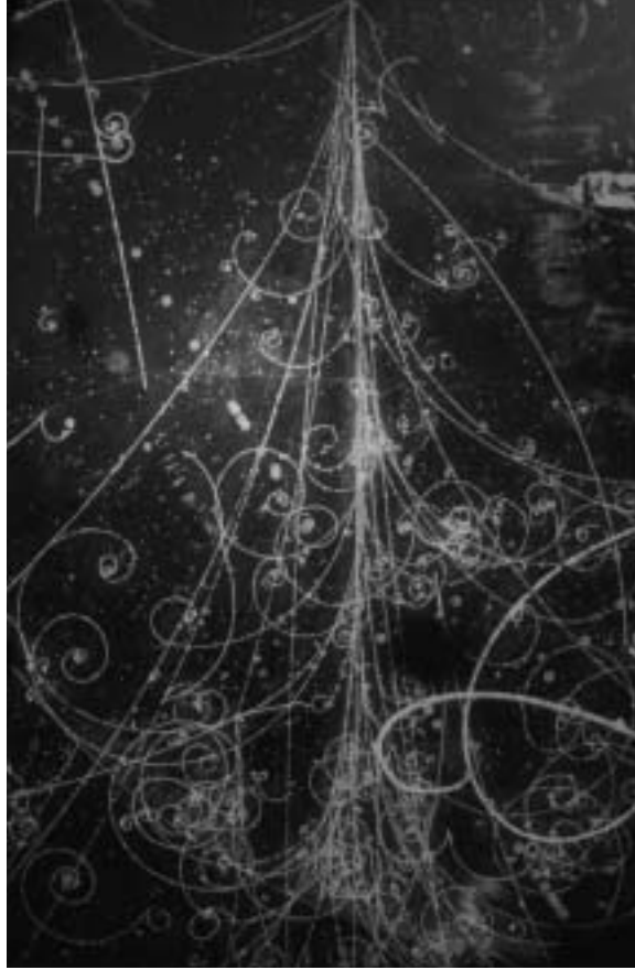
FIGURE 9.16 Trajectories of a burst of elementary particles in the magnetic field inside a bubble chamber.
