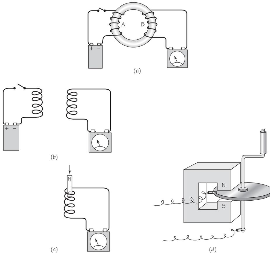
FIGURE 11.3 Various ways of producing electromagnetic induction.
