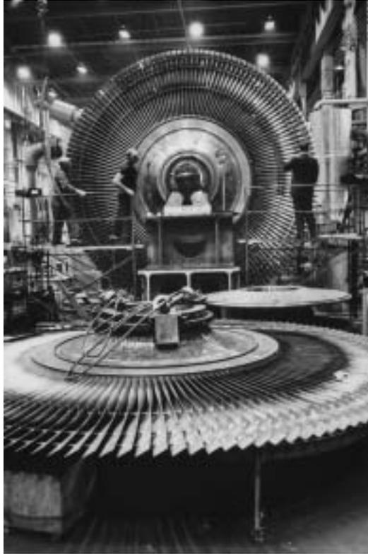
FIGURE 11.10 Steam turbine rotors.
