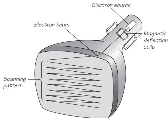
**FIGURE 12.12** Schematic diagram of a TV picture tube.
