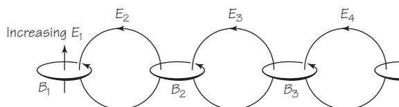
**FIGURE 12.5** Electric and magnetic fields linked by induction. An increasing electric field at the left (or current) surrounds itself with a magnetic field. As the current changes, it induces an interlinking electric field. The chain-like process continues with finite velocity. This is only a symbolic picture of the process, which propagates itself in all directions in space.
