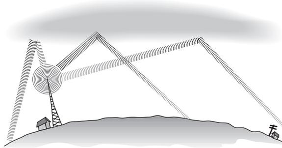
FIGURE 12.10 Radio waves bouncing off the ionosphere.
