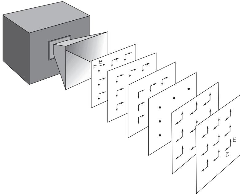
**FIGURE 12.6** In a microwave oscillator, which you may see in your laboratory work, electric oscillations in a circuit are led onto a rod in a metal “horn.” In the horn, they generate a variation in electric and magnetic fields that radiates away into space. This drawing represents an instantaneous “snapshot” of almost plane wave fronts directly in front of such a horn.
