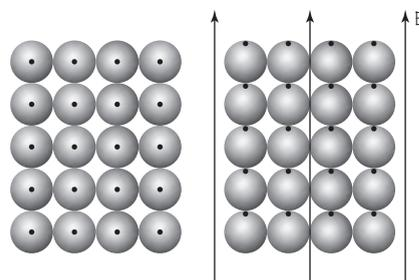
**FIGURE 12.3** When an electric field is set up in an insulating material (as in the diagram here), the positive and negative charges, which are bound to one another by attraction, are displaced. This displacement forms a current (the positive charges are represented by dots, and the negative charges by shaded circles).
