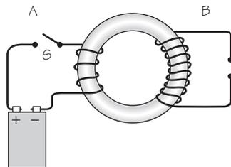
**FIGURE 12.7** Operation of the induction coil: Starting and stopping the current in coil *A* with a vibrating switch *S* produces a rapidly changing magnetic field in the iron core. This rapidly changing field induces high-voltage peaks in the many-turn coil *B* and can cause a spark to jump across the air gap. Spark coils for use in car engines operate this way.
