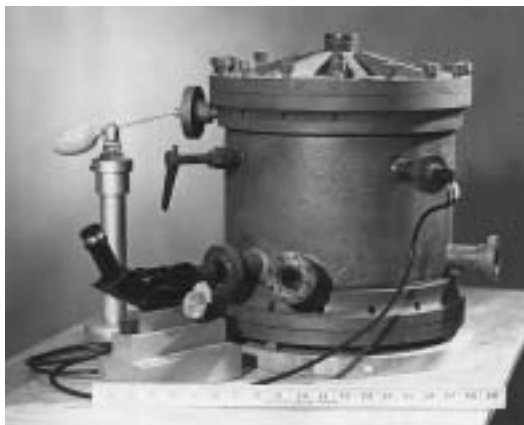
FIGURE 13.7 The original apparatus used by Robert Millikan to conduct his oil-drop experiment.
