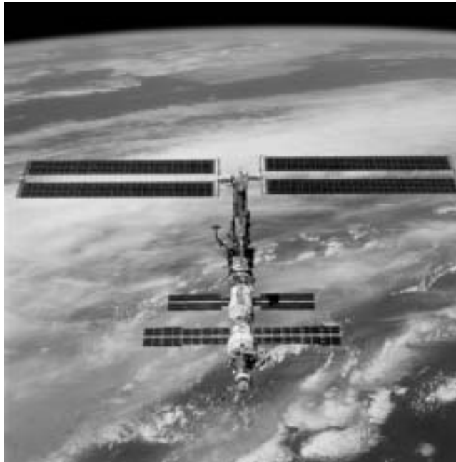
FIGURE 16.16 Artist's conception of International Space Station with its "wings" of photovoltaic cells.
