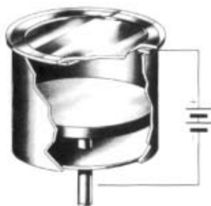
FIGURE 18.1 Cutaway drawing of the Wilson cloud chamber. When the piston is moved down rapidly, the gas in the cylinder cools and becomes supersaturated with water vapor. The water vapor will condense on the ions created along the path of a high-energy charged particle, thereby making the track. For his invention of the cloud chamber, C.T.R. Wilson (1869–1959) of Scotland shared the 1927 Nobel Prize in physics with Arthur H. Compton.
